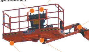
Jib boom and basket rotate allow additional functionality and access to hard to reach positions
